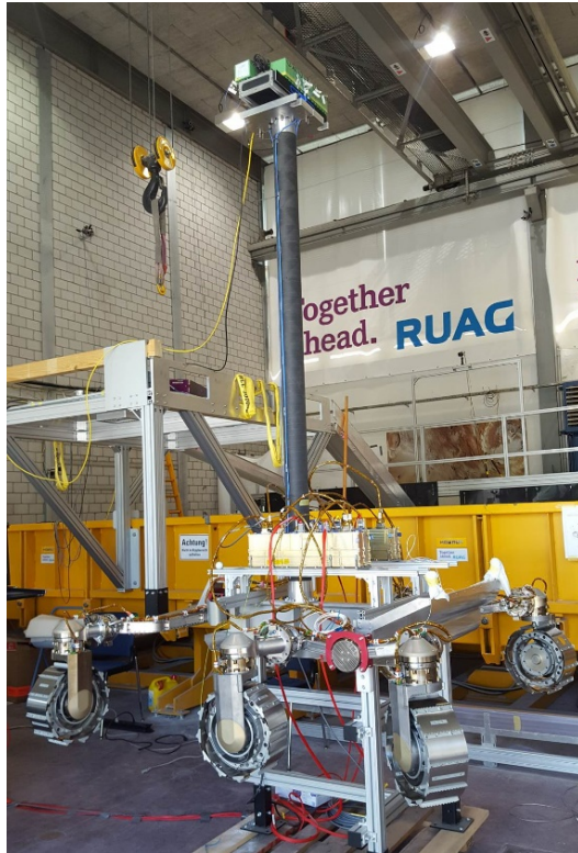
Rover chassis testing credit: RUAG-CH facilities
