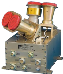
Solar CR Monitor
