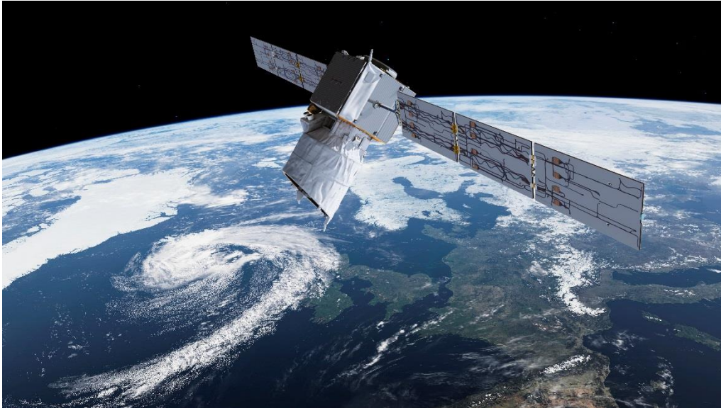
Fig. 6: ESA's ADM-Aeolus wind mission (planned launch 2017) will provide timely and accurate profiles of the world's winds and further information on aerosols and clouds. (Copyright ESA/ATG medialab)
