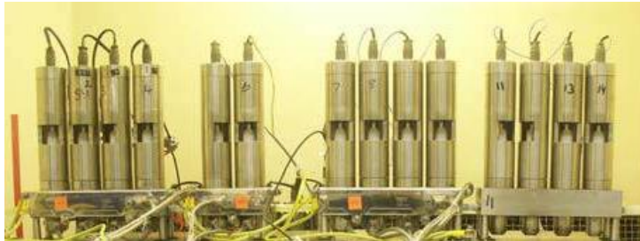
Centrifugal contactors performing extraction of Am241 from Pu solution.
