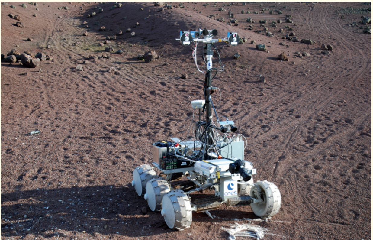
Three of ESA's ExoMars instrument prototypes are carried on this IARES rover model during tests, simulating the search for places to drill on Mars. ESA will provide the ExoMars rover for the 2018 mission.
